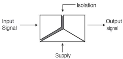
Figure: 2-way input isolation
