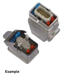
Example of coding option (6) of 16 different codings possible (4 coding pins per each connector coupling)
